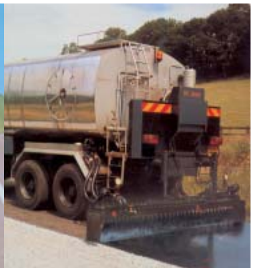
Cold-binding-agent spraying machines and vehicles with spraying ramps
