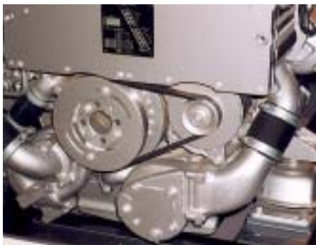
Installation cooling water pump KZTM
